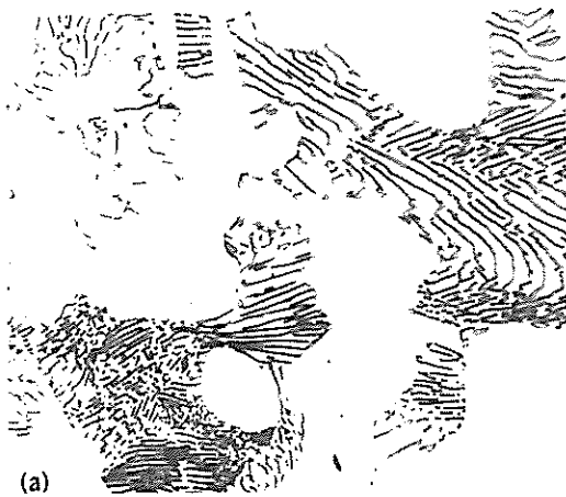
1030: Microstructures. (a) Picral, 1000x. Austenitized at 925 °C (1695 °F), 1 h; then 775 °C (1425 °F), 2 h 40 min; held at 710 °C (1310 °F), 4 h for isothermal transformation of austenite; brine quenched. Ferrite and coarse pearlite. (b) Picral, 1000x. Austenitized at 800 °C (1475 °F), 40 min; held at 705 °C (1300 °F), 15 min, for isothermal transformation; reheated to 710 °C (1310 °F), held 192 h. Partly spheroidized pearlite. Ferrite matrix
