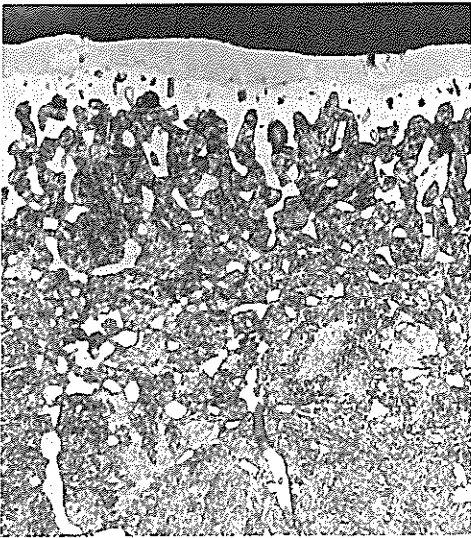
Microstructure of the case of a borochromtitanized construction alloy steel
