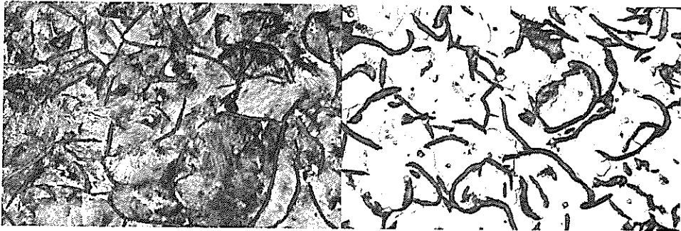
Microstructures. Structure of class 35 iron, as-cast (left) and after annealing
