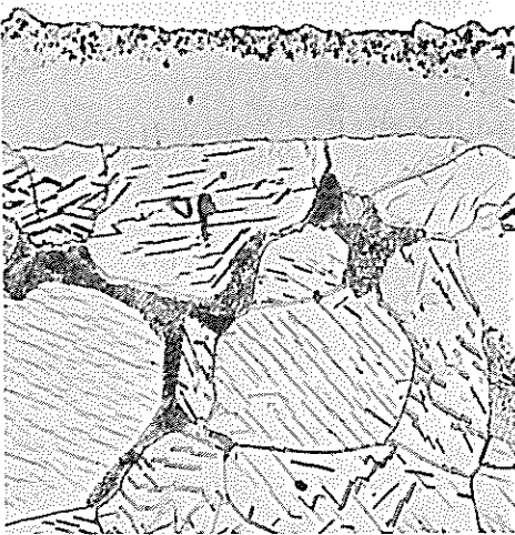
Nitrided case and diffusion zone produced by cyanide-cyanate liquid nitriding. The characteristic needle structure is seen only after a 300 °C (570 °F) aging treatment.
