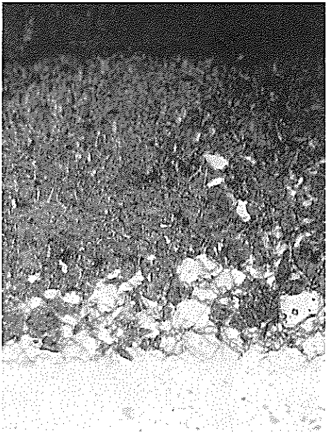
Observable diffusion zone on the unetched (white) portion of an ion-nitrided 416 stainless steel. Nital etched. 500×
