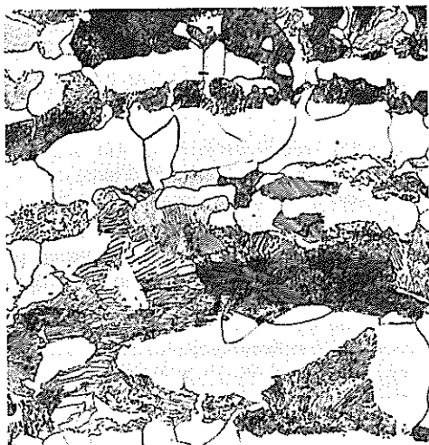
1040: Microstructures. Effect of prior microstructure on spheroidizing a 1040 steel at 700 °C (1290 °F) for 21 h. (a) Starting from a martensitic microstructure (as-quenched). (b) Starting from a ferrite-pearlite microstructure (fully annealed). Etched in 4% picral plus 2% nital. 1000x
